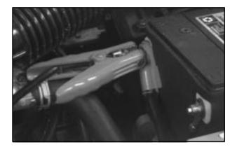
6. Remove the terminal cover and connect the red positive (+) cable to the positive (+) terminal of the dead battery. Use a remote positive (+) terminal if the vehicle has one.
